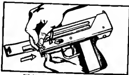
FIG. 10 Removing Pin Securing Receiver Group
